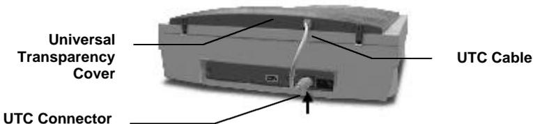
2. Plug the UTC cable connector into the round three-pin DIN connector on the scanner’s back panel.
